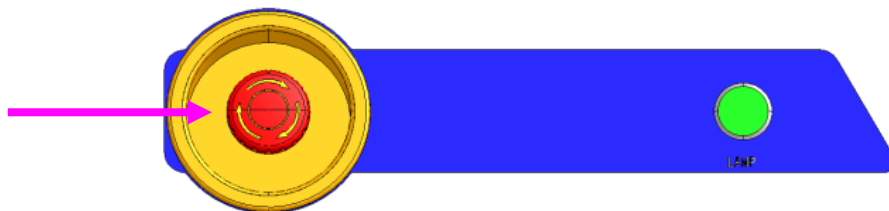
Emergency stop switch (EMO)
